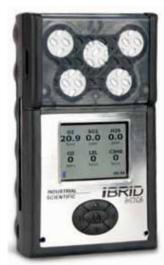
And a color display is more than eye-catching. It allows the user to step through instrument settings and functions with an intuitive menu and the instrument's five-way navigation button. It even supports the option of on-board graphing for easily interpreted direct readings and recorded data.
