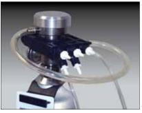
18105924 - 5-port Clamp-on Gas Manifold (I)
