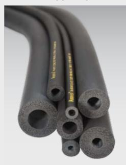
AEROFLEX-ECE is a special polymer based closed cell elastomeric thermal insulation especially developed to meet EN Standard (building material fire test standard). Aeroflex-ECE is classified as low flame spread, low smoke density and no flaming droplets according to EN 13823 & EN ISO 11925-2.
