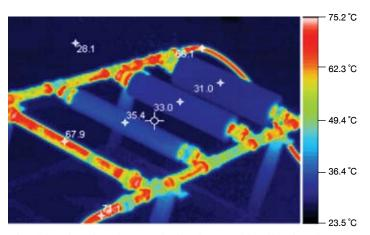
Infrared photo shows thermal energy emitted from hot water piping without thermal insulation and with various thickness of insulation, illustrating less thermal energy emittance from thicker insulation.
