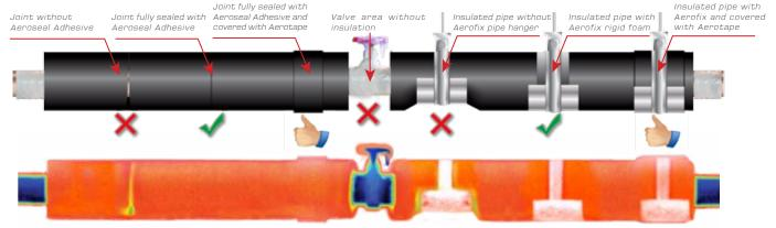
Fig. 5 The illustration shows the do and don't when installing Aeroflex insulation on low temperature pipeline to prevent condensation.
