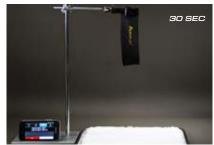
PE. Foam: this plastic insulation is manufactured from polyethylene plastic with tiny cells containing butane or similar gases, making the density approx. 2 lb/ft3. Most PE Foam insulation is highly combustible and can cause rapid flame transfer. It will melt and generate flaming balls (fire balls), causing flame transfer to other materials in buildings such as ceilings, carpets, and furniture.
