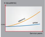
Low water vapor transmission, low water absorption and durability of material are very important factors for maintaining insulation properties during service, especially used in cooling system, EPDM based insulation has excellent durability, so Aeroflex is more stable in thermal conductivity (K value), less water absorption and less moisture penetration than other insulations that are made of NBR/PVC.
