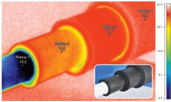
Infrared photo shows thermal energy emitted from low temperature nine without and with various thickness of Aeroflex thermal insulation. If surface temperature of insulation below dew point. condensation occurs.
