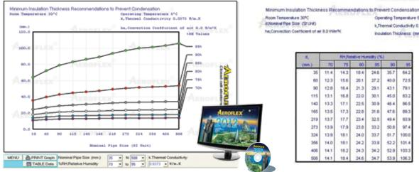
Fig. 2 Minimum insulation thickness recommendation graph and data table shows Aeroflex insulation thickness required to prevent condensation at various %RH and various pipe sizes. Aeroflex calculation program also calculates energy loss & gain, economic thickness and other calculation for HVAC&R industry.
