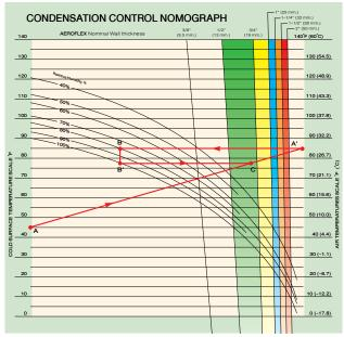
Fig. 1 Condensation Control Nomograph is a convenient tool for determining insulation thickness to prevent condensation.
