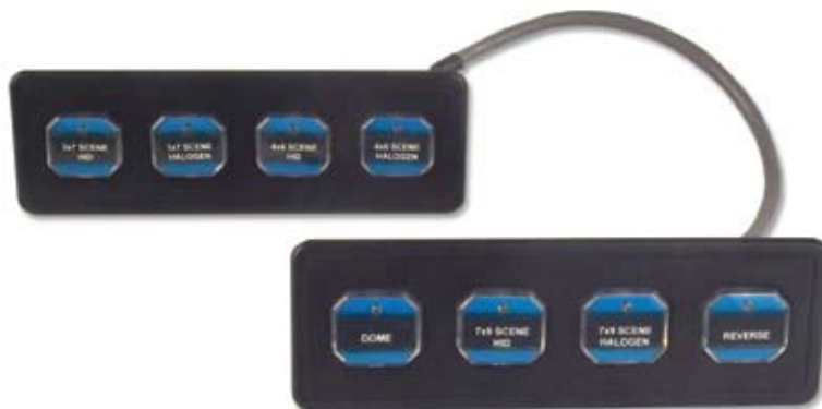
Two 3611-0400-00 connected with OL40-2020-00 cable assembly
