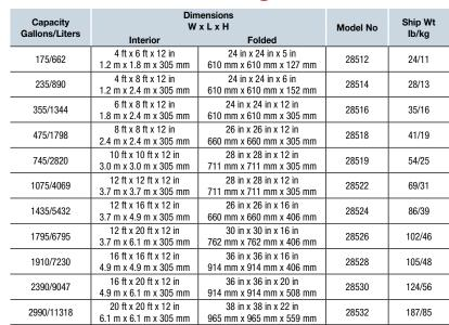
Note (1): For exterior dimension, add 8-in (203-mm) to width and length to account for support and hub. Note (2): When selecting a berm size, allow 12-in (305-mm) at entry or exit for lowering and raising the wall.
