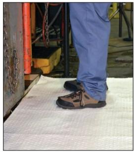
Use sorbent rolls to clean up workstation floors and reduce potential accidents.
