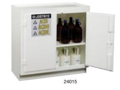
excellent chemical resistance to handle the most corrosive chemicals. A protective, all-welded bottom sump and a clean, sleek design complement any laboratory setting. Fully welded, liquid-tight 2-in (51-mm) sump contains accidental spills and makes clean up a snap. Shelf on larger units adjusts on 3-in (76-mm) center. Door accepts a padlock for security.
