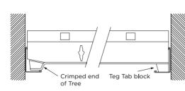
Cut, then form end with 6mm or 10mm crimping tool to suit depth of rebate on ceiling
