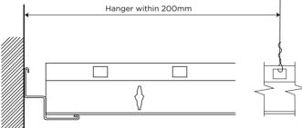
MS3600 Shadowline trim fixed to the perimeter wall, max 600mm centres as for standard trim
