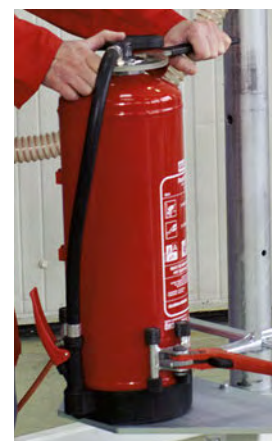
Universal chucking device to hold portable extinguishers during assembly
